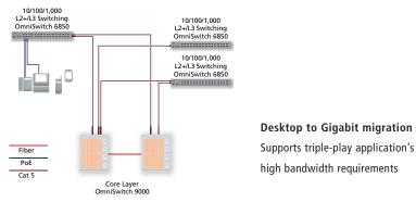
The OmniSwitch 6850s are ideal for use at the edge because of their compact fixed form factor design suitable for closets. Their modular expandability, flexible configuration provides an easy path to scale any workgroup up to 384 10/100/1000 ports and 16 10GigE ports in a single stack to support campus wiring closet requirements.
