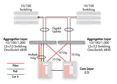
L3 Aggregation/Distribution Provides fiber or copper configuration options
